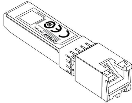
The AXM765v2 SFP+ module is a low-power, high-performance, 10GBASE-T transceiver. The AXM765v2 delivers 10 Gb network connectivity with cabling up to 262.5 feet (80 meters) of Category 6a (Cat 6a) or Cat 7 Ethernet cable.
